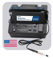
emission heated diode with audible and visual leak rate indicators. It is the most sensitive and accurate leak detector to detect all CFC, HFC and HCFC refrigerants as low as 0.006 oz/yr, including R-410a and R-507. The unit is mounted in a durable carry case which houses the 4.5 foot probe with built in filter, carrying strap, wall adapter and operating instructions.
