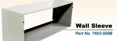
Our 42" wall sleeve is constructed from galvanized steel and powder coated for durability and aesthetic appeal. The wall sleeve comes factory assembled by spot welding to minimize breaches in the cabinet surface. It contains four chassis mounting holes, four grille mounting holes and two drain holes for optional drain kit.
