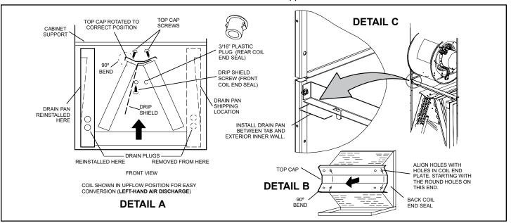
Figure 5. Field Modification for Left-Hand Discharge
