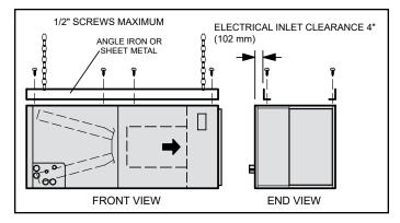
Figure 3. Suspending Horizontal Unit
