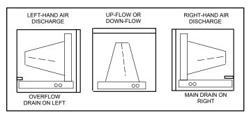
Figure 8. Main and Overflow Drain Locations Based on Coil Orientation
