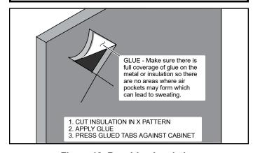
Figure 12. Repairing Insulation
