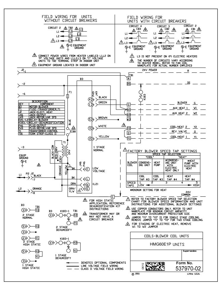
Figure 11. Typical System Wiring Diagram
