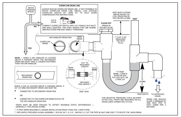
Figure 7. Typical Main and Overflow Drain
