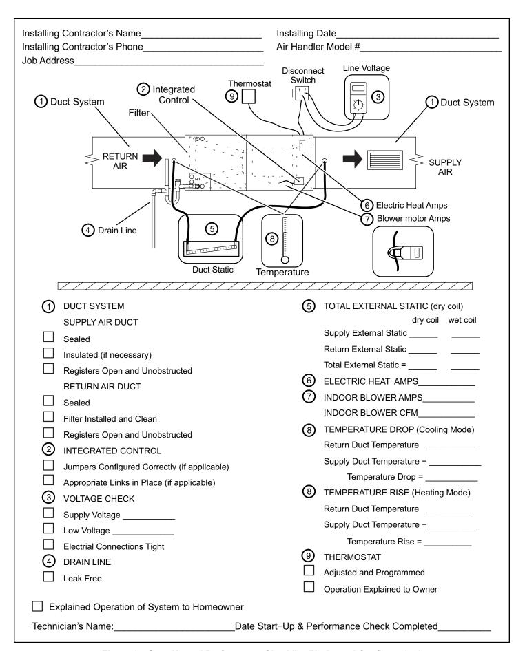
Figure 14. Start-Up and Performance Checklist (Horizontal Configuration)
