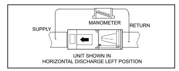
Figure 9. Static Pressure Test
