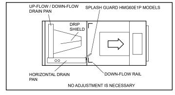
Figure 2. Right-Hand Discharge Configuration
