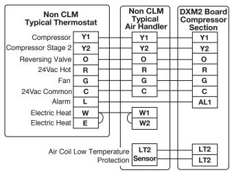
**Note:** Air coil low temperature protection will not be active if LT2 sensor is not installed or is not installed correctly.
