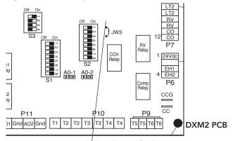
JW3-LT1 jumper should be clipped for low temperature operation. Do not clip JW3-LT1 in open loop applications
