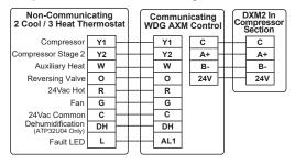
When a non-communicating thermostat will be used to control the system a Comfort-Aire/Century 7602-457 thermostat must be connected so that proper system communications and operation are maintained. The 7602-457 may be installed at an inconspicuous location near the air handler and wired to the TB1 terminal strip of the AXM control board. The 7602-457 should be set to the OFF mode.
