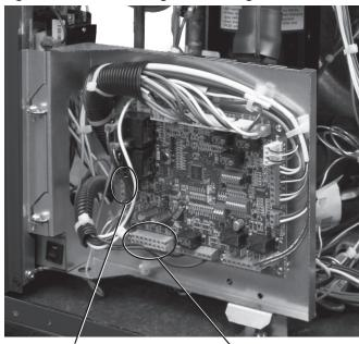
Low Voltage Field Wiring When Using Digital Air Handler
