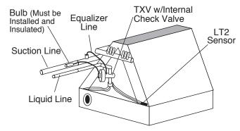
**IMPORTANT:** DO NOT perform any brazing with the TXV bulb attached to any line. After brazing operations have been completed, clamp the TXV bulb securely on the suction line at the 10 to 2 o'clock position with the strap provided. Insulate the bulb and line with pressure sensitive tape.
