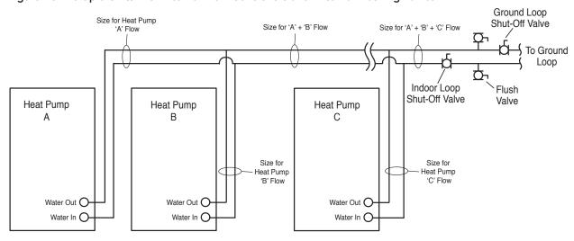
First, flush the ground loop. The installer should close the indoor loop shut-off valve (or the internal flushing valves in all units) and open the ground loop shut-off valve to prevent flow through the indoor loop while flushing the ground loop.
