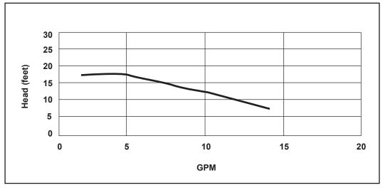
Figure 6b: High Head 25-140 Internal Flow Controller Pump Performance
