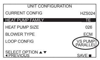
Installer Settings System Config Unit Config Loop Config
