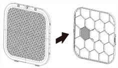
Separate the frame from the filter assembly.
