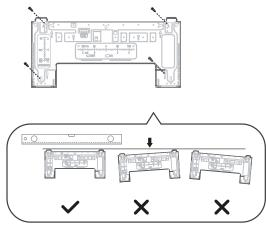
Correct orientation of Mounting Plate
