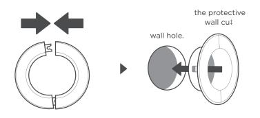
Place the protective wall cu<sup>‡</sup> in the hole .
