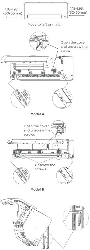
Use the holder at the back of the unit against on the mounting plate to prop up the unit
