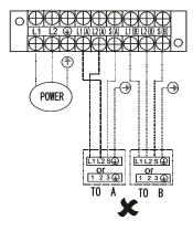
**NOTE:** For quick-connector models, please refer to <<USER MANUAL >> packed with the indoor unit. Refer to the following figures if end-users wish to perform their own wiring. Run the main power cord through the lower line-outlet of the cord clamp. ---- This symbol indicates field wiring.
