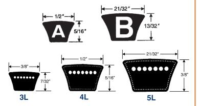
Various shaped belts have long been used for industrial power transmission, including round and flat shaped belts.
