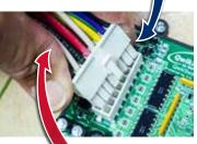
16-pin Connector from Motor to Qwik**Swap**® Board
