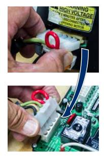
5-pin Connector from Motor to Qwik**Swap**® Board
